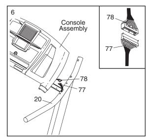
7. Set the console assembly on the Handrail (20). Be careful to avoid pinching any of the wires. Hand tighten five Screws (3) into the Handrail and the console assembly. Do not put Screws into the two indicated holes. Start all five Screws, but do not tighten them yet.
